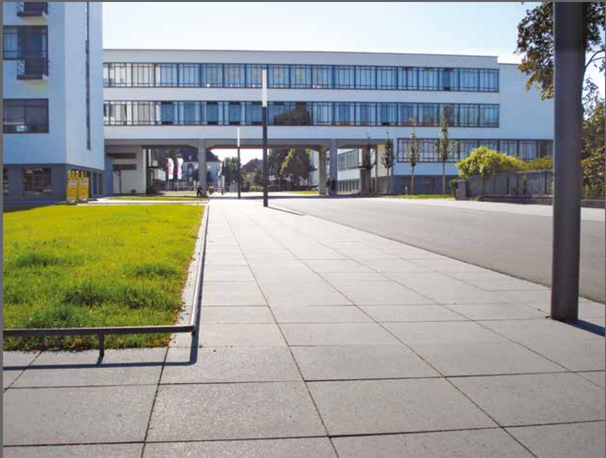
60 x60 City-Truck pavings and a special paving including recesses for edgings (see technical drawing)
